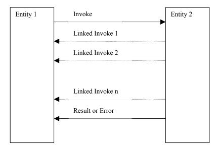
In this diagram, Entity 1 "invokes" Entity 2 by sending an Invoke message. This Invoke message contains a set of standard fields (the header) and an application-specific body. This is a fully encoded ASN.1 message component. Entity 2 responds with a set of one or more optional Linked Invoke messages (which themselves can be encapsulations of the entire described protocol) followed by a final Result or Error message (these too can be optional but are usually included).
