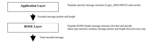
On the decode side, the process would be reversed with the message flowing up the stack:
