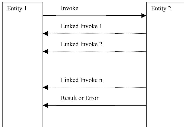
In this diagram, Entity 1 “invokes” Entity 2 by sending an Invoke message. This Invoke message contains a set of standard fields (the header) and an application-specific body. This is a fully encoded ASN.1 message component. Entity 2 responds with a set of one or more optional Linked Invoke messages (which themselves can be encapsulations of the entire described protocol) followed by a final Result or Error message (these too can be optional but are usually included).
