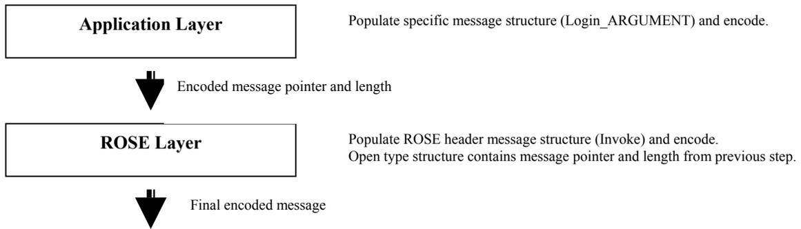
On the decode side, the process would be reversed with the message flowing up the stack:
